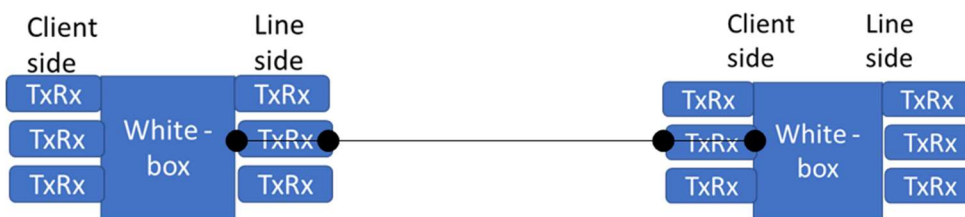
Figure 2-2 IP link provisioning between the whiteboxes.
