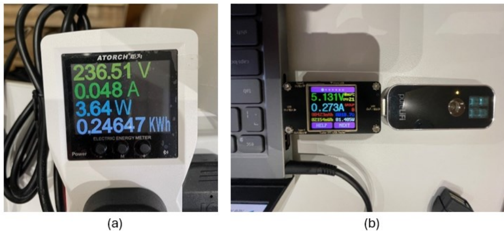
Figure 3-3: Measured power consumption: (a) LiFi AP; (b) User dongle.
