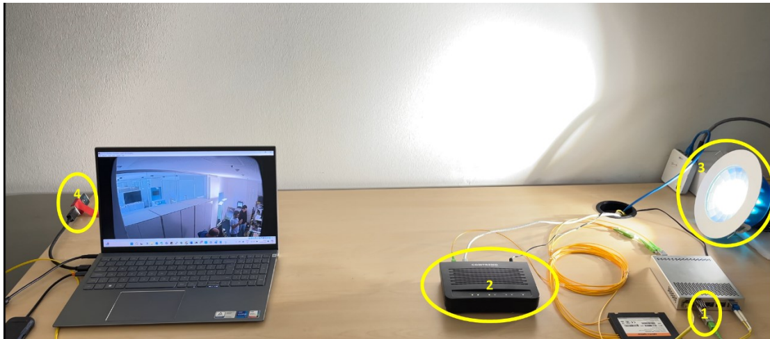
Figure 4-5: the setup of LiFi over PON including (1) the Tibit OLT, (2) the ONU, (3) the LiFi AP, and (4) the LiFi USB dongle.
