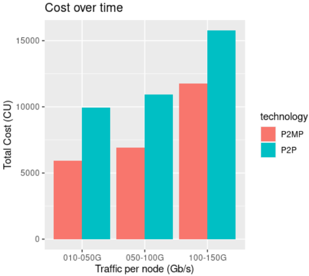
Figure 56 Total cost evolution in the short and medium term for 1,000 nodes: P2MP vs P2P technology.
